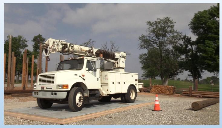
The candidate will stow the boom, raise the outriggers and return the DD to "road ready" condition. The DD is then secured.
