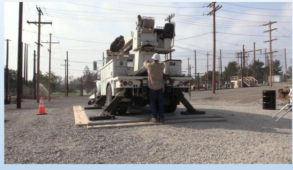
The candidate will then start the digger derrick, properly set the outriggers and level the machine.
