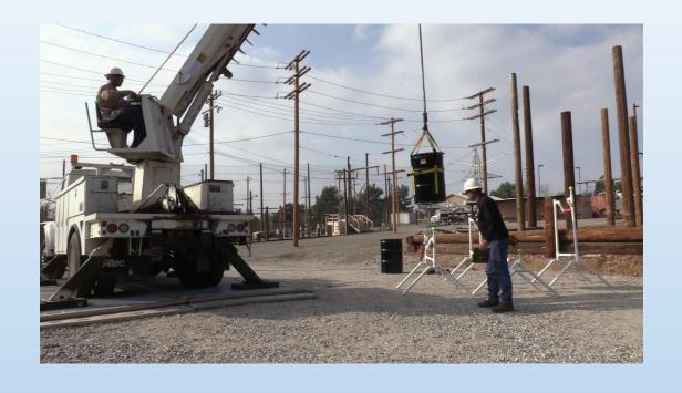
Raise and maneuver the load drum so that the line hose touches the red crossbar area of each goalpost. The route and order through the four goalposts is very specific. The line hose under the load drum is then positioned back into the open top barrel where the task began.
