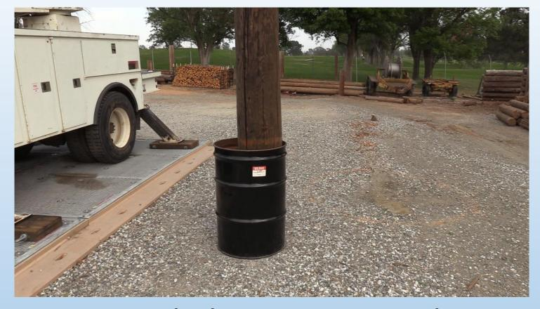
After the examiner helps to position the upright pole into the DD pole claws, the task will be to maneuver the pole so the butt is inside the open top drum about 12".
